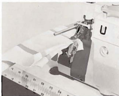
AIR FABRIC UNCURLER —This unit, designed for Class 39500 machines, uses air jets to remove curls from top and bottom plies of flat knit materials as fabric passes through sewing area. Style 2899 B-1
